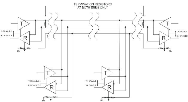
Figure A-1: Typical RS485 Two-Wire Multidrop Network
