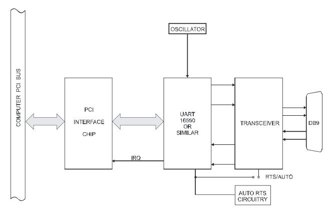
Figure 1-1: Block Diagram(Only one serial channel shown)
