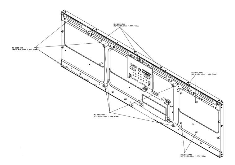
Note : 1.CN1:JAE FI-RTE51SZ-HF 2.CN2: JST S14B-PHA-SM3-TB(HF) 3.UNSPECIFICED TOLERANCE IS 0.8mm 4.TOQUE OF M3 USER HOLE:7kgf-cm MAX. 5.TOQUE OF M4 USER HOLE:10kgf-cm MAX. 6.TOQUE OF M6 USER HOLE:16kgf-cm MAX.
