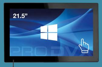
Industrial Grade (X86) Panel PC for Commercial usage. Sizes from 7 inch up to 32 inch. Plastic and Metal Housing.
