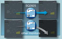
EIZO's fully automated stability function uses an internal backlight sensor to stabilize the brightness level throughout the life of the monitor, compensating for fluctuations caused by variations in ambient temperature and the passage of time.
