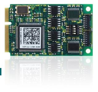
multitasking operating systems, reduce CPU utilization, and improve data throughput, while reducing or eliminating inter-character or interpacket pauses. The advanced integrated circuit with pre-scalar supports a wide variety of custom baud rates, and any rates not otherwise achievable can be supported via a custom factory-installed crystal oscillator (up to 10Mbps!).
