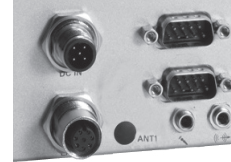
M12 railway power input and two Gigabit LAN connector
