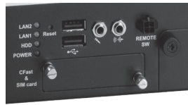
Removable CFast™, SIM slot and suspension 2.5"SATA HDD/SSD
