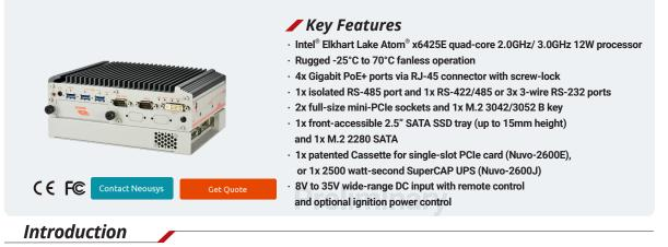
The Nuvo-2600 series is an Intel<sup>®</sup> Elkhart Lake Atom<sup>®</sup> fanless box-PC with flexible expansions to fulfill versatile factory automation and machine vision applications that require a compact footprint, Gigabit PoE+ capability, and front-accessible data storage with CPU performance at 12W of low power consumption.
