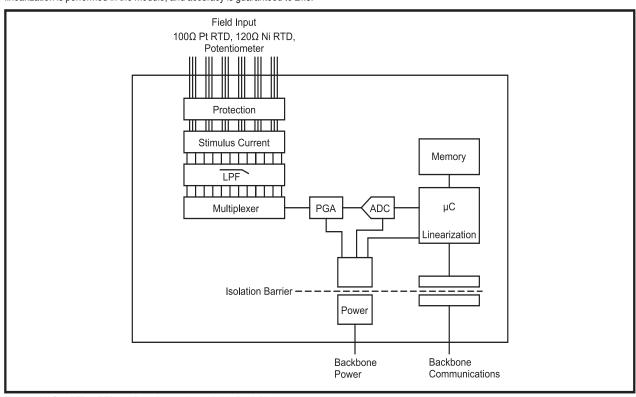
Figure 1: MAQ20-RTD31 RTD and Potentiometer Input Module Block Diagram
