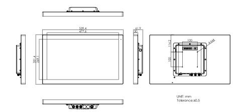
21.5" FHD IP66/IP69K stainless steel display, VGA/HDMI input, OSD on the rear side, projected capacitive touch, 9~36V DC power input with Adapter 21.5" FHD IP66/IP69K stainless steel display, VGA/HDMI input, OSD on the rear PhanTAM-121APH side, projected capacitive touch, 9~36V DC power input with Adapter, 1,000 nits LCD
