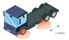
It is recommended that sensors on rigid vehicles and articulated tractor units have coverage six metres down the nearside or one metre from the rear of the vehicle (or tractor unit), whichever is smaller.
