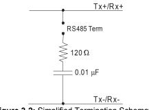
Figure 3-2: Simplified Termination Schematic
