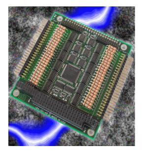
The 104-IDI-48 family boards are 48-channel PC/104 utility boards which feature 48 individually optically isolated digital inputs. They are ideal for use in control and instrumentation applications where high voltage protection is required. Individual channel-to-channel isolation allows every channel to be physically and electrically separated from the others.
