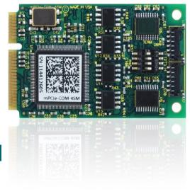
multitasking operating systems, reduce CPU utilization, and improve data throughput, while reducing or eliminating inter-character or interpacket pauses. The advanced integrated circuit with pre-scalar supports a wide variety of custom baud rates, and any rates not otherwise achievable can be supported via a custom factory-installed crystal oscillator (up to 10Mbps!).
