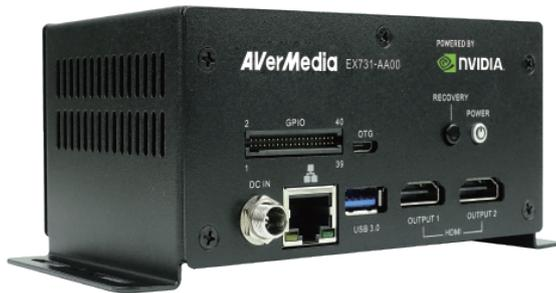
AVerMedia EX731-AA00-2AC0 Box PC equips NVIDIA® Jetson™ TX2 module to provide a compact design with dimension W: 117.2mm x L: 76.8mm x H: 61.0mm (4.61" x 3.02" x 2.4" with mounting ears W: 144.8mm, 5.7")
