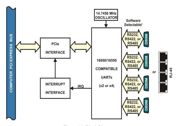
Figure 1-1: Block Diagram
