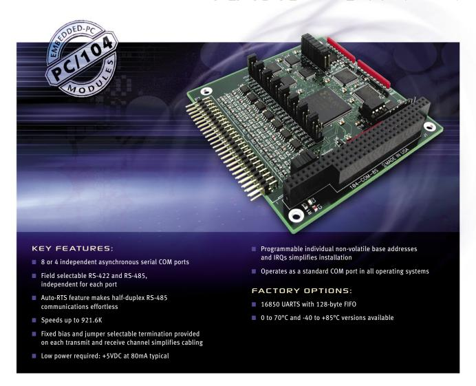
The 104-COM-8S and 104-COM-4S are eight and four port, asynchronous, serial communication boards that support both RS-485 and RS-422 communications. Ideal for POS, gaming systems, machine monitoring, military, and high-density networking applications, these boards may be installed in any system with PC/104 support. Ports are accessed via a 50-pin IDC type right angle connector.
