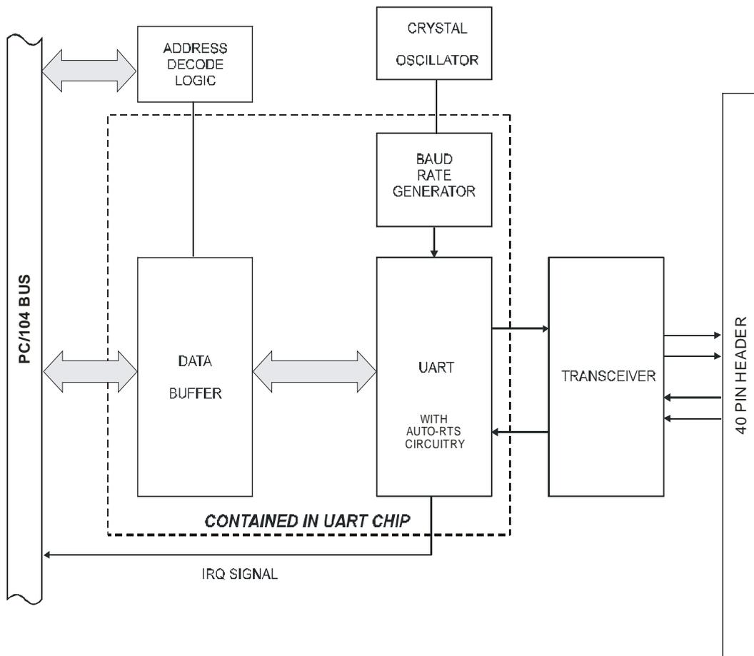
**Figure 1-1: BLOCK DIAGRAM**
