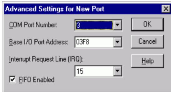
To add a COM port, use START|CONTROL PANEL|PORTS applet and click ADD, then enter the correct UART address and Interrupt number.
