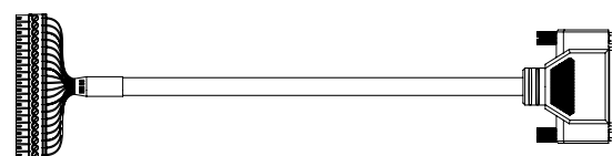
Figure 2: 8B Backpanel Interface Cable
