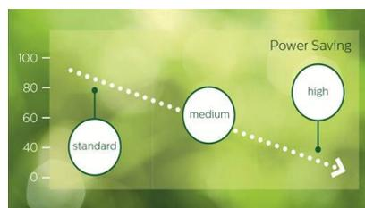
The backlight intensity can be controlled and pre-set by the system to reduce the power consumption by up to 50%, which saves substantially on energy costs.
