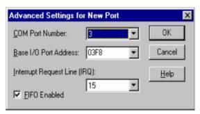
To add a COM port, use START|CONTROL PANEL|PORTS applet and click ADD, then enter the correct UART address and Interrupt number.
