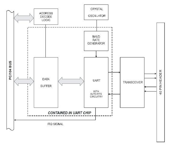
Figure 1-1: BLOCK DIAGRAM (Only one serial channel shown)
