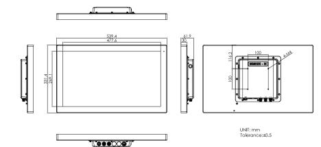
21.5" FHD IP66/IP69K stainless steel display, VGA/HDMI input, OSD on the rear side, projected capacitive touch, 9~36V DC power input with Adapter 21.5" FHD IP66/IP69K stainless steel display, VGA/HDMI input, OSD on the rear PhanTAM-121APH side, projected capacitive touch, 9~36V DC power input with Adapter, 1,000 nits LCD
