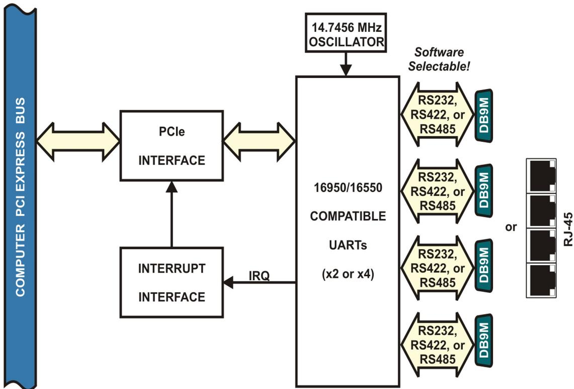
**Figure 1-1: Block Diagram**
