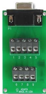
Figure 1-2: ADAP9 Screw Terminal Accessory
