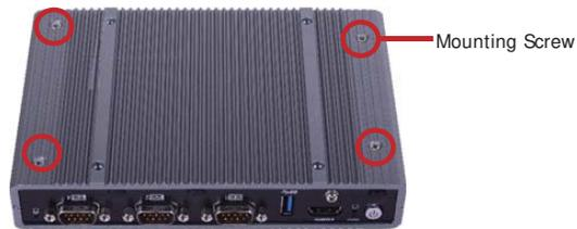
4. After removing the mounting screws, lift the cover up.
