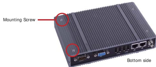
2. Align the mounting holes of the system and the mounting holes on the bracket, and then use the screws removed on step 1 to secure the bracket in place.
