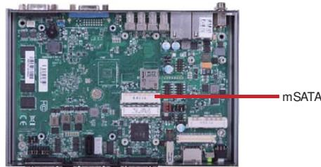
2. The system board is equipped with a mSATA slot. The mSATA slot supports full length mSATA card. Note the key on the slot. The key ensures the mSATA card can be plugged into the slot in only one direction.
