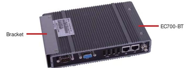
3. The 3 mounting holes on the bracket of the system is used to mount the DIN rail bracket.
