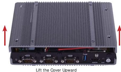
5. The 3 Mini PCIe slots, the microSD socket and the HDD bracket are readily accessible after removing the bottom side of the chassis cover.
