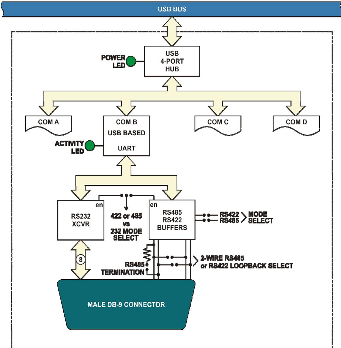
Figure 1-1: Block Diagram (Only one full serial channel shown)
