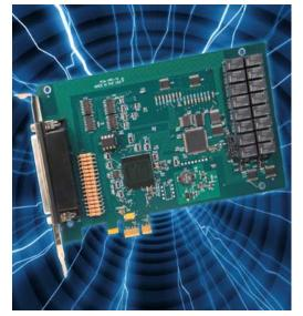
DC and are not polarity sensitive. Input signals are rectified by a diode bridge and applied to the inputs of opto-isolators. A 1.8k ohm resistor in series provides current limiting. Standard 12/24 AC control transmitter outputs can be accepted as well as DC voltages. The input voltage range is 3V to 31VDC (or 40-10kHz RMS). To extend the input voltage range, you may connect external resistors in series.
