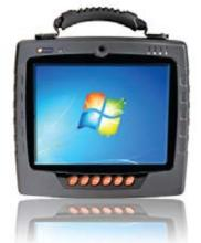
The DLI 8500P vehicle Mount Terminal combines wireless communications, GPS, and mobile computing in a single portable device suited to a variety of industrial applications including:
